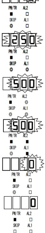
③To stop the buzzer sound, press RESET switch. In this occasion, alarm light changes to steady light and it becomes self reset mode. To decrease reading below alarm level with DOWN switch, alarm light and alarm contact are cancelled.
